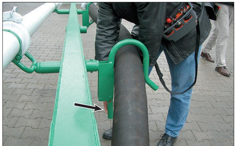
**Fig. 7.17 Release the discharge hose**
