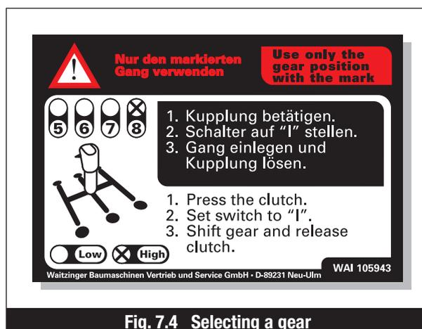
Fig. 7.4 Selecting a gear
