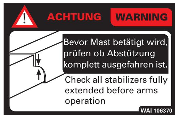
Fig. 2.30 Item 14 - WAI106370 - Fully extend the outrigger
